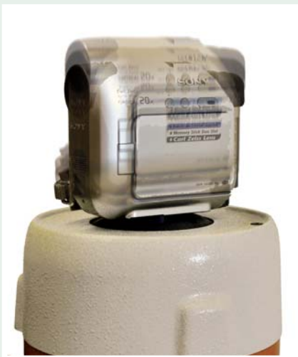
V406 shaker being used to test camcorder to ensure product reliability during operation.
