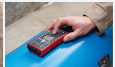
Tests for rotation direction on a running motor with the built-in noncontact, wireless sensor – specifically important for fast running motors or motors where the shaft is not visible.
